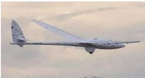
The Airbus Perlan 2 aircraft has set a new altitude world record for a glider, climbing to 52,172 feet. This new record was set on 3rd Sept 2017 at El Calafate in Argentina. The Perlan 2 is a composite intensive engineless glider designed to fly at the edge of space using stratospheric mountain waves. The aircraft soared to an incredible 52,172 feet without the help of engines. The earlier record was held by Perlan 1 which had climbed to 50,727 feet in 2006.
